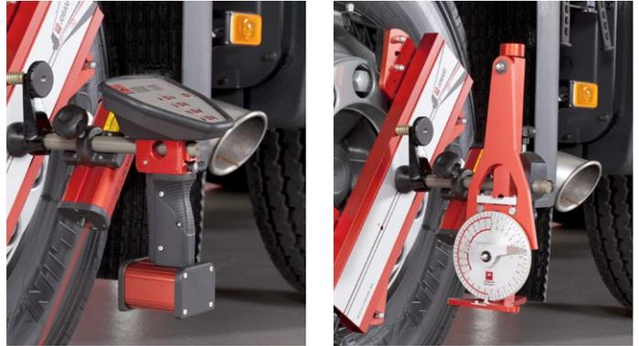
*There are two gauges available for measuring camber, caster and KPI: electronic (left) and analog (right).*
