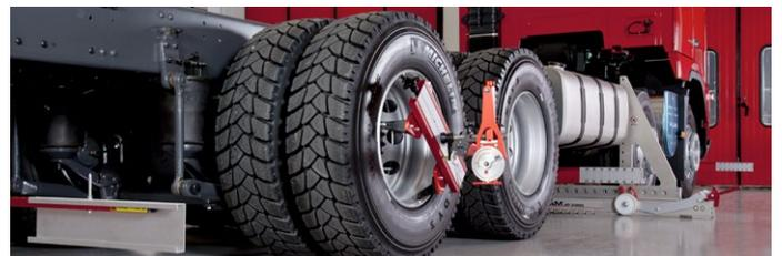
JOSAM laser AM can easily be configured to measure chassis frames. This is possible with additional frame gauges, a supplementary software or special report sheets. A frame check is part of every alignment procedure.
