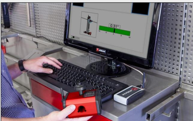
The camera based calibration is an extension for the JOSAM cam-aligner system. Measurements are calculated and displayed in the accompanying software. Reports are printed from the PC.
