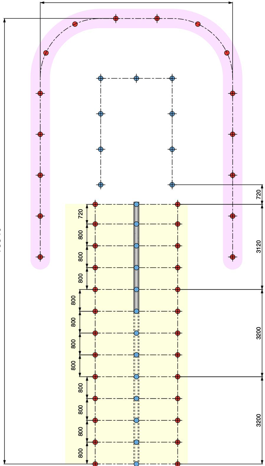
JOSAM i-press 9.6 meter in combination with high pulling function. The working place covers a total area of 16340 x 7000 mm.
