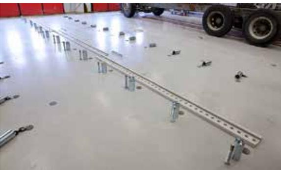
JOSAM i-press is anchored in a centre beam and floor anchorings that are included in the equipment. This kit covers a workplace of 9.6 x 3 m. It can easily be extended with sections of 3.2 m.
