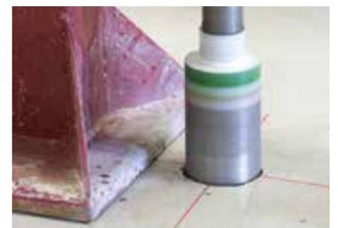
If the workshop would like to do frame straightening by using the floor anchoring expander solution JOSAM i-press with a centre beam then the following drawing is available:
