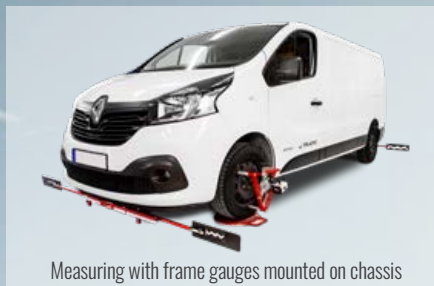
Measuring with frame gauges mounted on chassis
